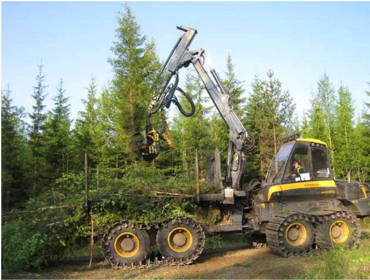
Picture 11. An energy harwarder is more profitable than a two-machine system at short forwarding distances or on small stands. (Photo: Juha Laitila)
